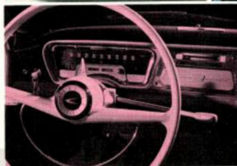
Heater & defroster, gear shift on steering column, turn indicators, dual-tone horns, key-turn power starting.
