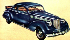
The Royal Rumble Seat Coupe 119 Inch Wheelbase . . . 95 Horsepower
