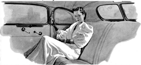
Foot rests are built as an integral part of the front seat and move backward and forward as a unit.
