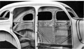
ALL-STEEL BODIES . . . Chrysler's steel all-steel bodies are built like a uniform, unperforated shell, and carry up to 20,000 pounds' equivalent weight, distributed over the length to provide the most rigid, solid body built. There are no holes or stressed points to cause flex.
