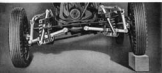
IMPROVED FRONT WHEEL SPRINGS ... are equipped with Chrysler's special coil, which gives more spring to provide a cushioned ride of spring action—both front and rear.
