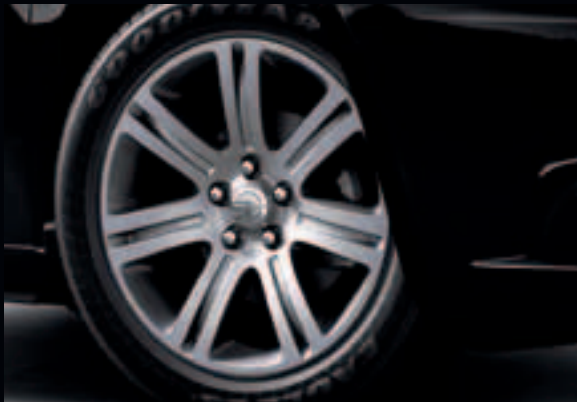
18-INCH CAST ALUMINUM WHEEL WITH PAINTED SATIN SILVER FINISH Optional on Touring.
