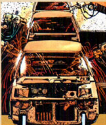
Robot welders provide precise welds.
