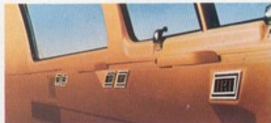
Auxiliary air conditioner/heater system is sidewall mounted. Club Wagon shown.
