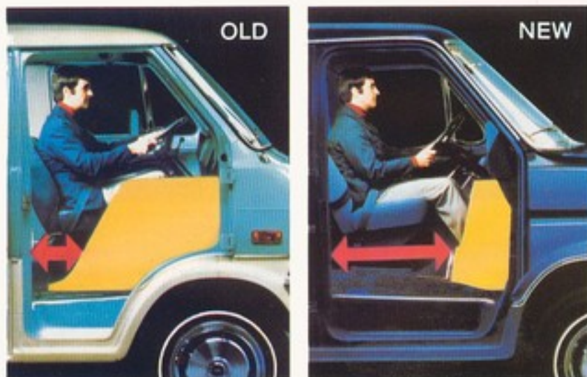
Engine, front axle and wheelhousings are all moved forward in Econoline '75. The relocated engine provides longer down-the-middle cargo area than in '74, gives the driver easier access to the load, creates new move-around room for driver and passenger.
