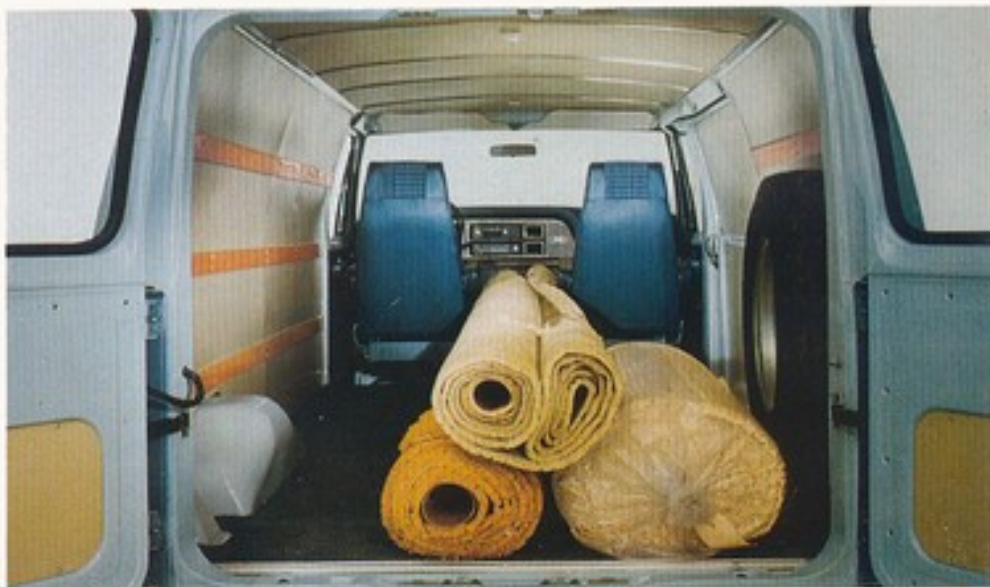
Rear opening is a full 54 in. wide, 10% wider than last year's Econolines. Slam-shut door design makes closing easy. Center cargo length is increased 12 in. Captain's Chair's shown, optional.
