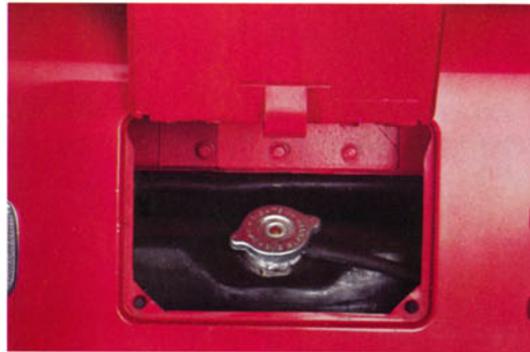
Water is checked through a spring-loaded hinged door on front of the cab. Radiator cap is angled for convenient filling. Every service operation is made just as easy as possible.
