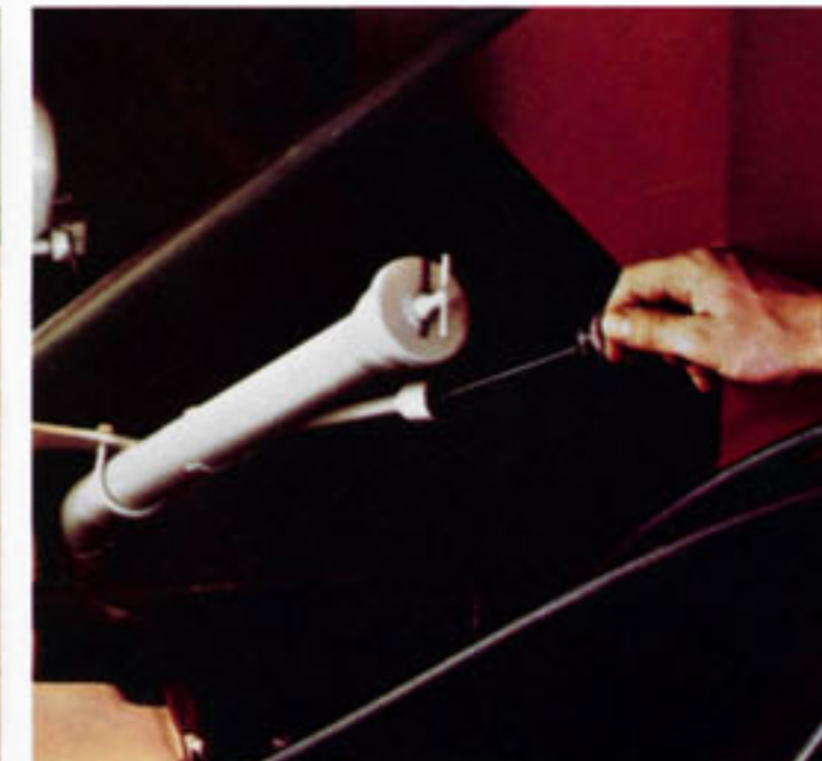
Both oil dipstick and filler pipe extend from the engine to the back of the cab. You can check or add oil with cab in place.
