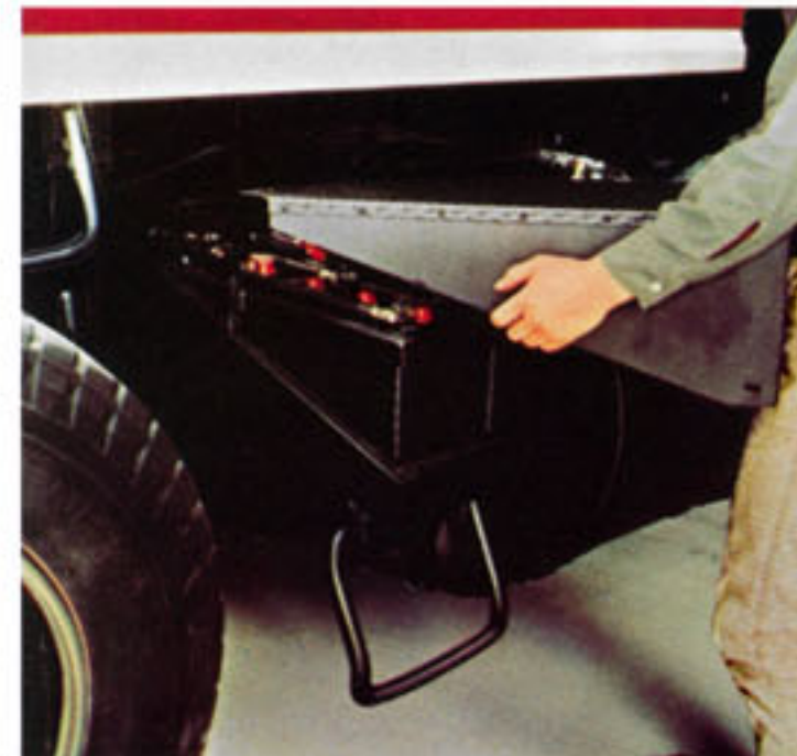
Batteries can be serviced without tilting cab. This handy arrangement encourages proper servicing, helps cut maintenance costs.
