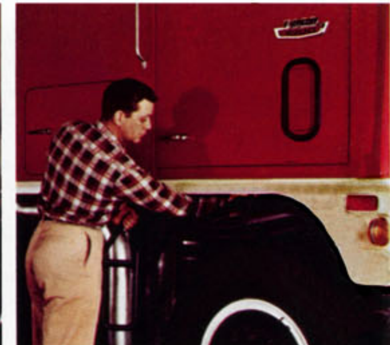
Draining Ford's under-floor air tanks is a snap. Just reach under the cab skirt and open the pet cocks. No other truck makes this job so easy.
