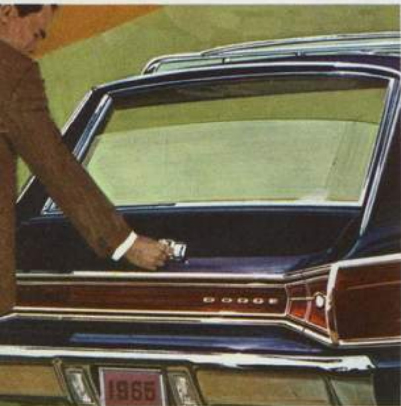
Dash switch or tailgate key controls rear window electrically. Children cannot control window from inside.
