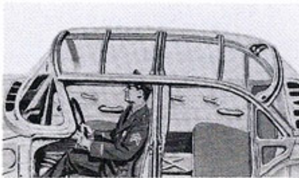
EXTRA-RIGID ROOF SUPPORTS AND BRACES . . . New fluted roof panel is supported by 5 all-steel roof cross braces. In addition to giving reinforcement to the roof, they provide valuable passenger protection in case of roll-over.
