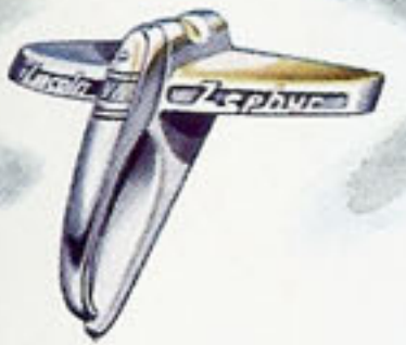
The license plate light is built into this handle, which turns to raise the rear deck.
