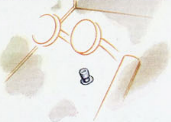
Bright headlights may be deflected instantly by pressing foot against the floor button. A red warning light shines imperatively on the panel when the high beam is on.
