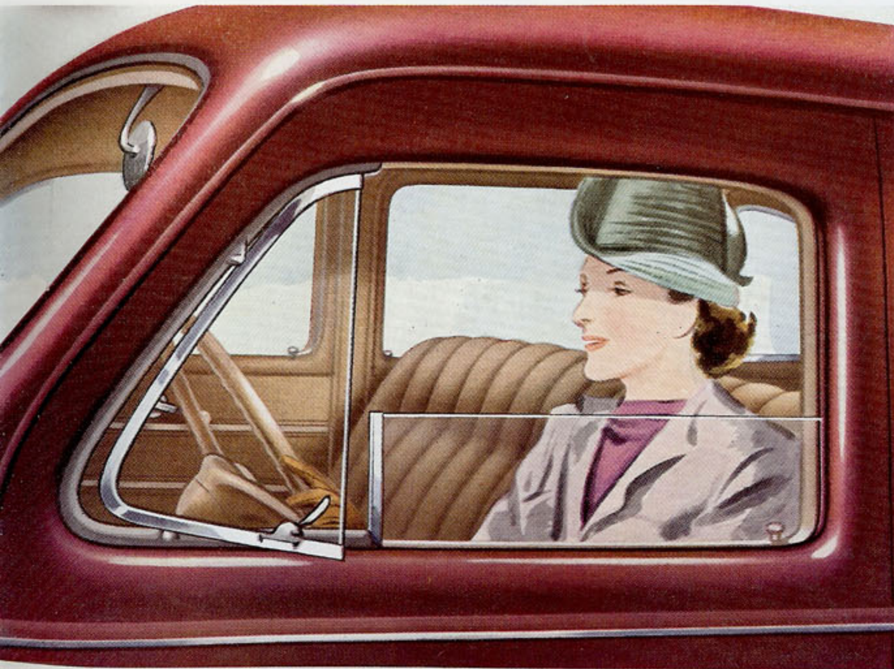
Ventilation is through new control windows built into the forward part of the front door windows and operating independently of door handles. Just open this ventilating window, and fresh air blows in without draft on those in the rear seat.
