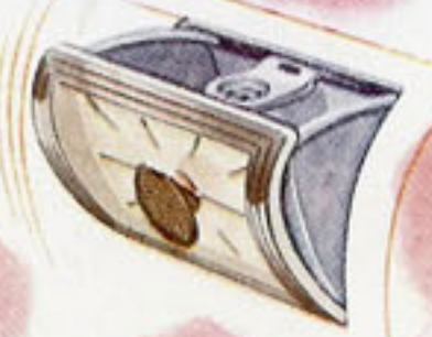
On the instrument panel is an ash receiver. On the panel, also, and in the rear compartment, is a snap-out type lighter.
