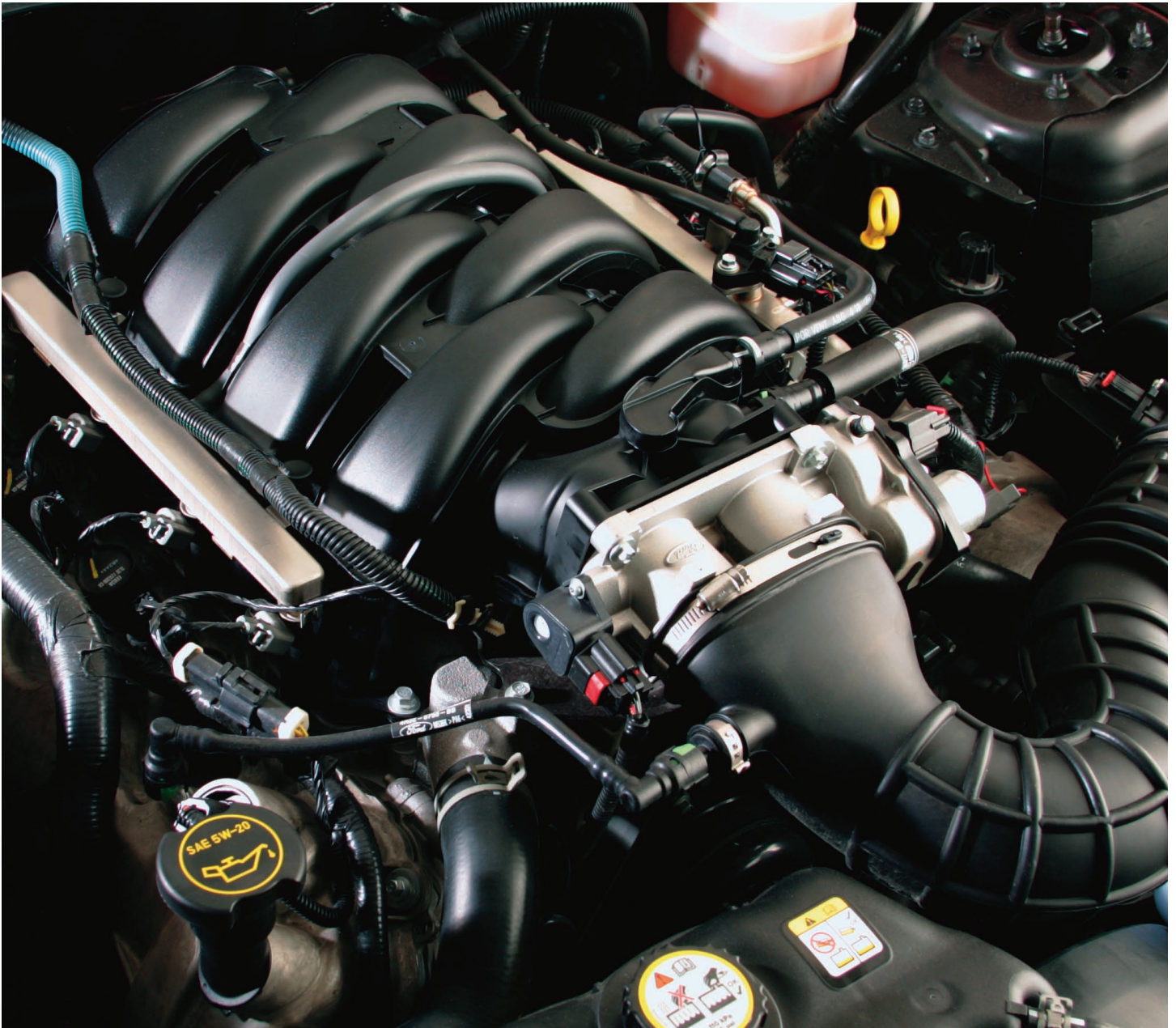
Mustang's 4.0L V6 offers 210 hp, while the 4.6L V8 (shown here and standard on every Mustang GT) matches 300 horses with 320 lb.-ft. of torque. Things get a bit more serious with the Shelby Cobra, though. Like 500 horses and 480 lb.-ft. of torque serious on its supercharged 5.4L V8.
