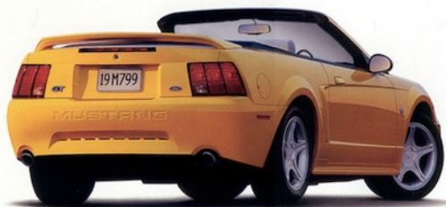
Mustang GT convertible in Chrome Yellow Clearcoat Metallic. The updated modular 4.6-liter single-overhead-cam V8 makes 260 horsepower with 302 lbs.-ft. of torque.
