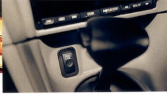
Located conveniently in the shifter bezel, the available Traction Control on/off switch puts enhanced traction within easy reach.
