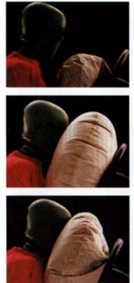
Shown here is a representation of a driver-side air bag Supplemental Restraint System deployment. The air bag inflates in less than one-tenth of a second in the event of a moderate to severe frontal impact, then deflates in a fraction of a second.
