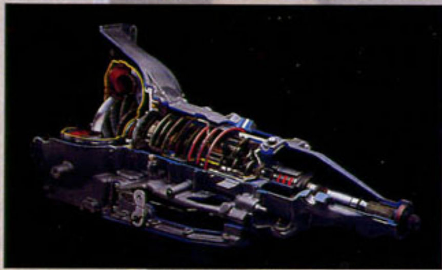
Town Car's automatic overdrive transmission lets the engine run slower at cruising speed, so it improves fuel economy.
