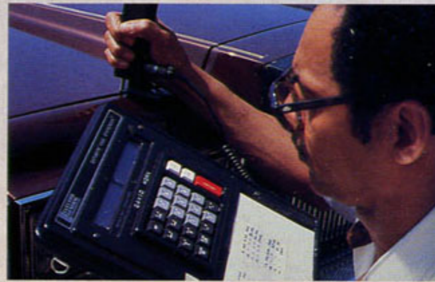
The fit between one body part and the next is evaluated by a computerized measuring device.
