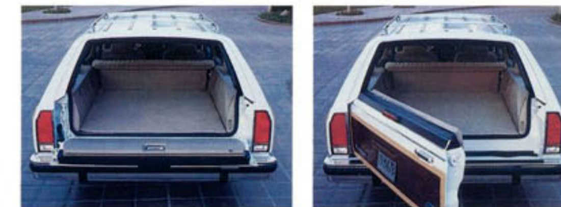
The 3-way doorgate, standard with wagon models, provides the necessary versatility to handle people- and/or cargo-carrying situations efficiently.
